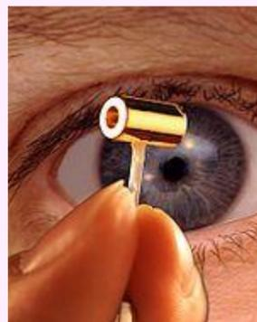
The 48 beams are focused to enter the hohlraum through a 2 mm hole on either end.
