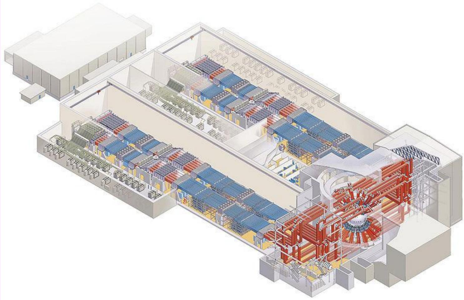
The NIF is a giant facility (which can be seen by scale of the people shown in it). It is three times larger than a football field. It is the most complex optical facility ever created. It is designed to produce altogether a 500 trillion-watt flash of light, precisely focused onto a target smaller than a pea, with the light arriving from 48 directions simultaneously, timed to within picoseconds.
