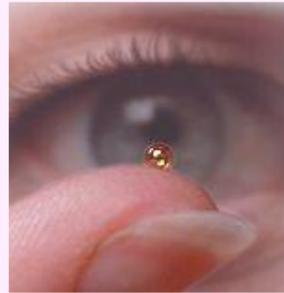
The fuel target is made up of a thin 2 mm wide shell of beryllium with a layer of solid deuterium-tritium deposited on its inner wall. The deposited fuel, weighing 0.238 mg, is frozen to minus 255 degrees Celsius. The above photo (a mockup) indicates the size of the target capsule.
